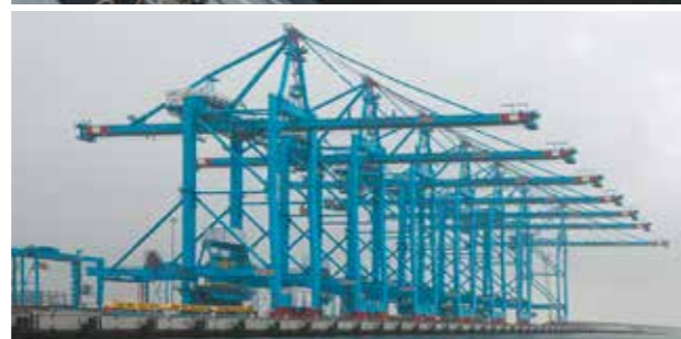
For the APMT Maasvlakte II terminal in Rotterdam, Kalmar delivered eight of the world's first remotely controlled extra-large "EEE" monobox cranes as well as two barge quay cranes.
