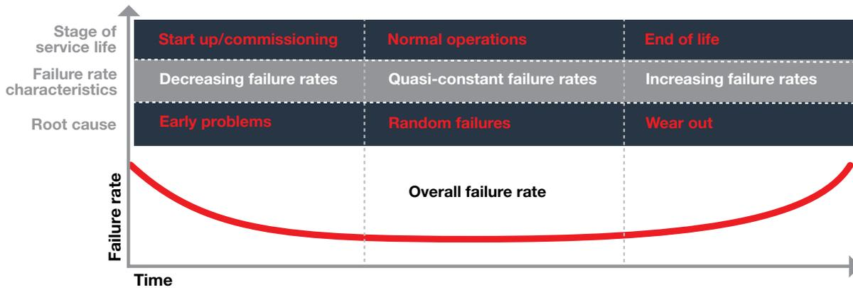
Failure rates begin at some non-zero level on start-up, decrease as the equipment and system are optimised, and then gradually rise again as the equipment nears the end of its planned lifetime.
